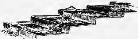
Fish ladders are a series of adjoining pools to help fish get past dams or falls.
